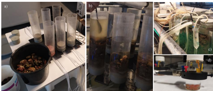
Fig. 1. The photos summarise the sequence of actions for the mesocosms apparatus and the measurements: a) preparation of the cores with spawning gravel, b) egg pocket construction and laying eggs, c) falcon tube sampled with the needle oxygen logger and d) chamber used to incubate eggs for the microcosm assay.
